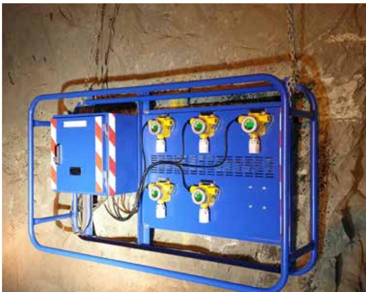
Another benefit of the monitoring solution is that it allows for quicker re-entry times and staged re-entry to the underground mine workings by eliminating the requirement for personnel to physically check that each level is clear before opening the workings. Re-entry times are already down by 10%.
